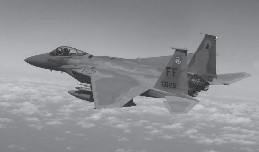
Figure 1.1 Aerodynamics is required for all components of the F-15E in flight, including the wing, fuselage, horizontal and vertical tails, stores, and how they interact with each other (U.S. Air Force photo by Staff Sgt. Samuel Rogers).
